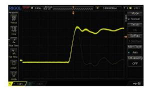
UltraVision: waveform recording and playback functions
