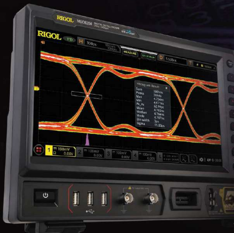
Perform eye measurement on the 622 Mb/s signal.
