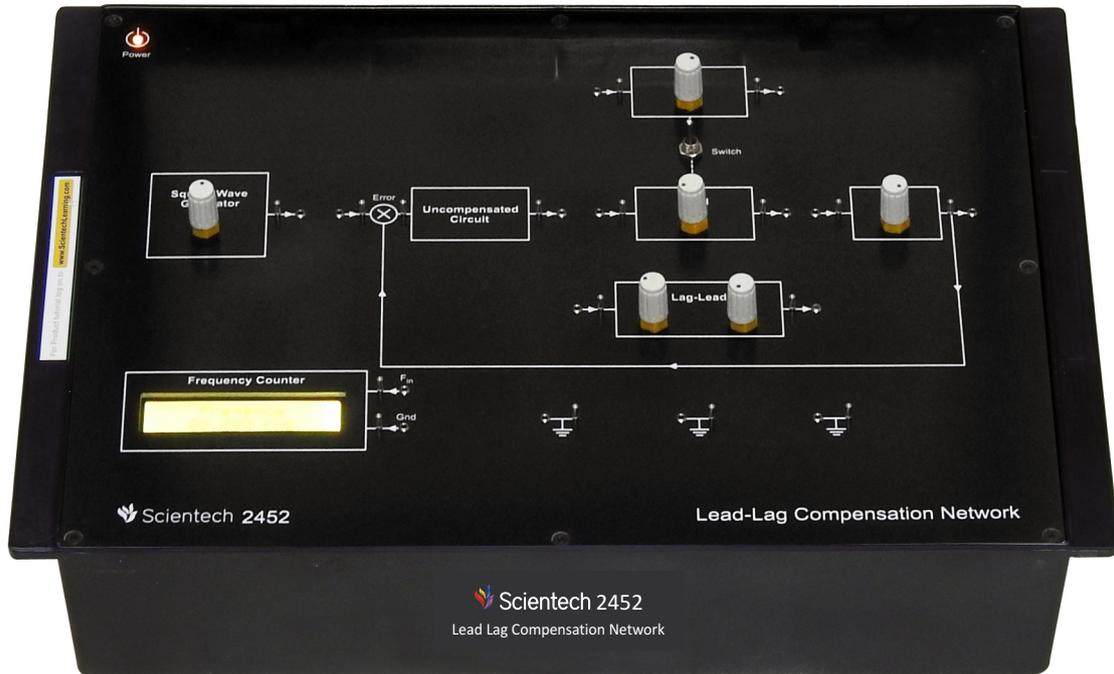
**Scientech 2452 is a Lead Lag Compensation Network** which helps the user to gain invaluable practical experience of the principles and application of Leading Lagging of a signal applied to any active network.
