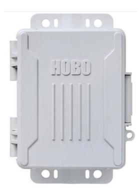
Rugged and compact, the redesigned HOBO USB Micro Station is a weatherproof data logger for multi-channel monitoring of microclimates. Starting at just \$240, this battery-powered station accepts up to five plug-and-play Smart Sensors and has a hinged door to make sensor installation simple and quick. The Micro Station is equipped with a built-in USB port for fast, efficient data readout to a computer, and integrated mounting tabs for easy installation.
