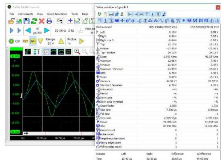
The measurement results are shown in a special value window that can be positioned anywhere on your computer screen. A convenient toolbar allows you to enable or disable a measurement with a single click. The measurement results can be copied to the clipboard e.g. to use them in reports. When printing the graphs, the cursors and measurements results are also included.
