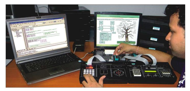
Input Interface module MC01 is an extension module for Nvis Microcontroller development platforms. The module has been designed for students and practicing engineers to gain invaluable practical experience on the principle and applications of microcontroller. The object is to have a clear understanding of how input peripherals are interfaced and controlled with microcontroller.
