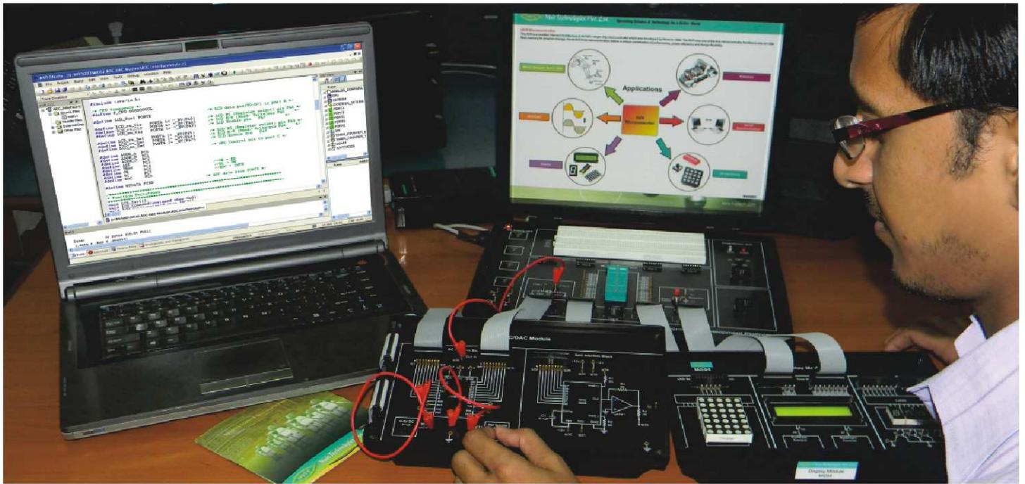
**ADC/DAC module MC02** enables the students and practicing engineers to gain invaluable practical experience on the principles and applications of microcontroller. The object is to have a clear understanding of how analog inputs are converted into digital through Microcontrollers and vice versa. ADC/DAC module, MC02 has inputs and outputs terminals for connection to external real world applications.
