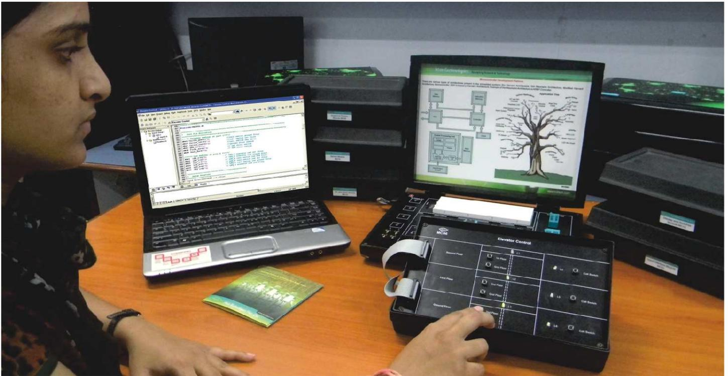
Elevator control module MC06 enables the students and practicing engineers to gain invaluable practical experience of the principles and application of Elevator and Microcontroller.
