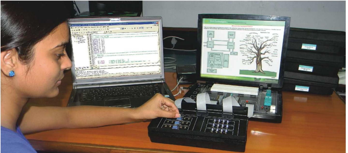
TTL I/O Interface module MC07 enables the students and practicing engineers to gain invaluable practical experience of the principles and applications of a Microcontroller.
