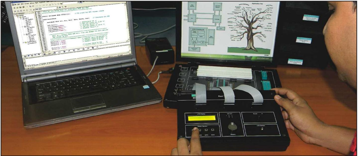
Real Time Clock module MC08 is an extension module for Nvis Microcontroller development platforms. It helps the user to gain invaluable practical experience of the principles and application of real time clock, LCD, switch and buzzer module in microcontroller based projects.
