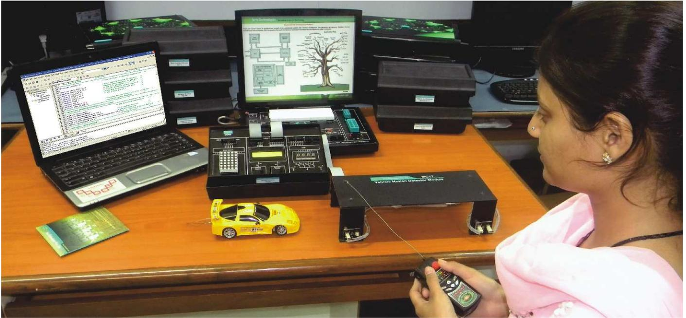
Nvis Technologies Vehicle motion detector module, MC17 is an extension for Nvis Microcontroller development platforms. The object is to have a clear understanding of how to measure the speed of vehicle using Microcontroller. Vehicle motion detector module. MC17 has input and output terminals for connection of external real world applications.
