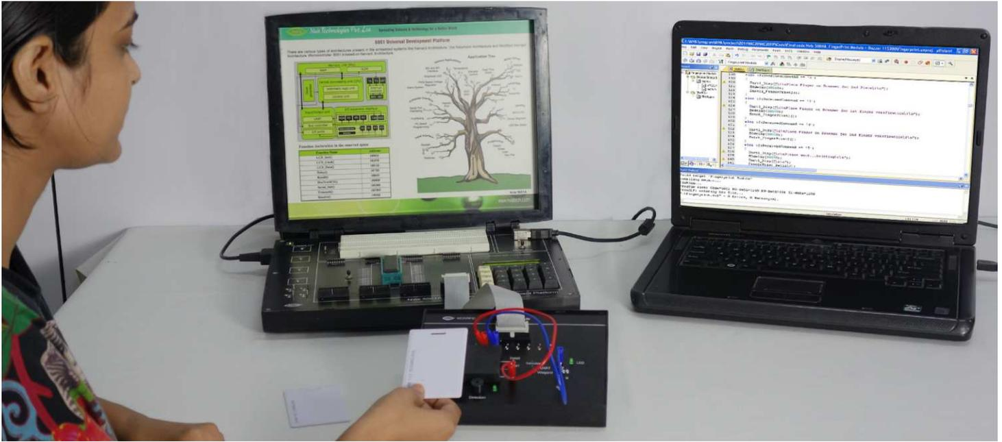
**RFID Card Reader Module MC20RFID** is an extension module for Nvis Microcontroller development platforms. The module has been designed for students and practicing engineers to gain invaluable practical experience on the principle and applications of microcontroller & RFID card reader. The objective is to have a clear understanding of how RFID card reader is interfaced and controlled with microcontroller.
