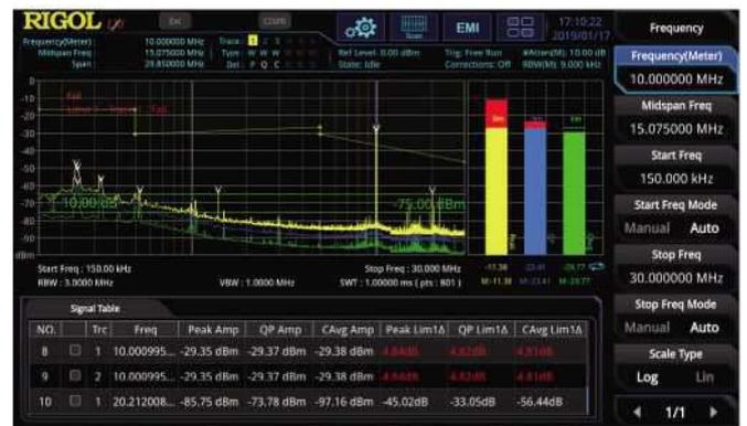
Quickly recall the limit line compliant with the CISPR standard (e.g. EN55011, EN55012, etc.) to carry out pre-test and monitor the target point with three different detectors.
