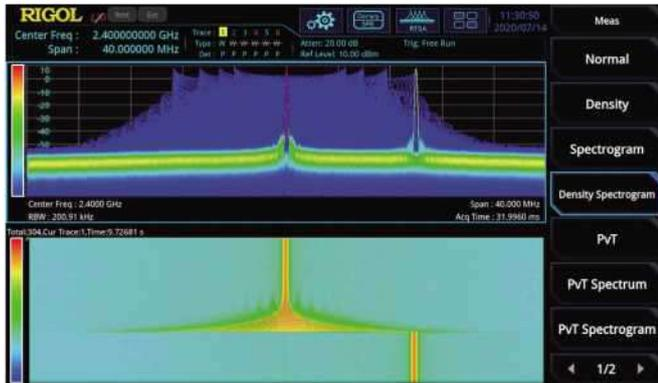
Density spectrum for you to visualize how frequently signals occur
