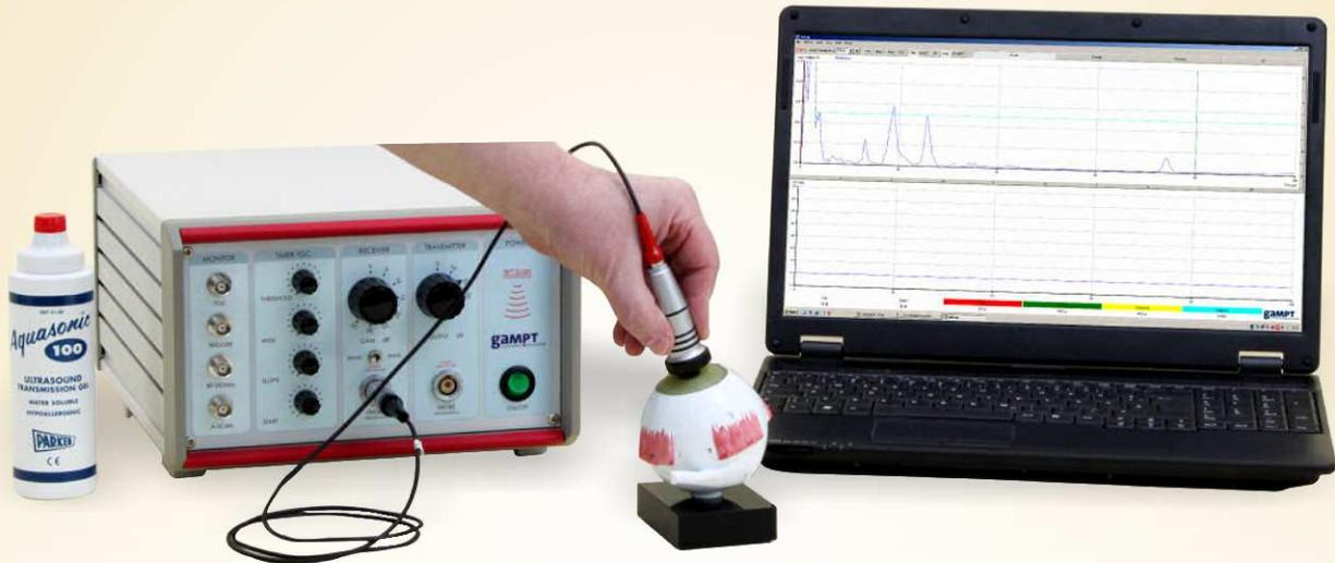
**Ultrasound Eye Dummy Scientech 11E** is used in ophthalmology (ophthalmology is a method for diagnosis of diseases in the eye.) for measurement of distance of Retina and Cornea. The distance between Retina and Cornea is measured by A-Scan Mode. By using A-Scan mode we can also measure depth of Retina and Cornea and also do analysis of thickness of lens.
