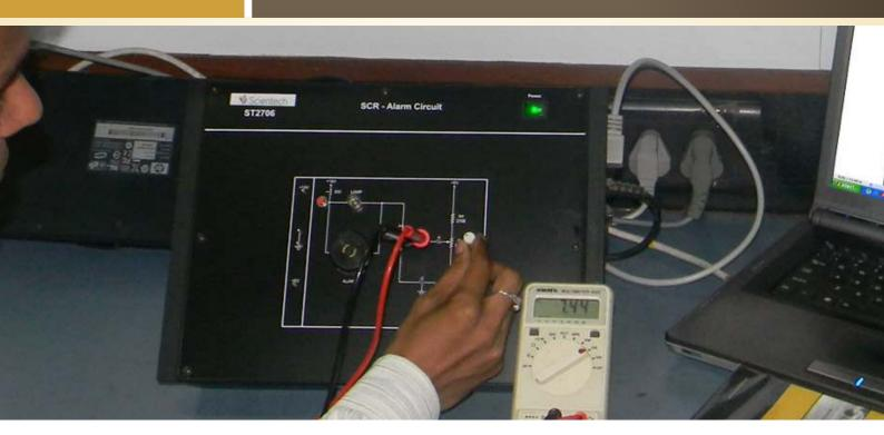
Scientech 2706 is a platform which is very useful Students to understand the low voltage application of the SCR in alarm control. 2706 is provided with the built in power supplies, sockets for making different interconnections in the circuit and exhaustive learning material.
